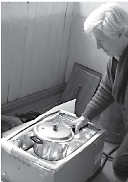
Figure 5: The pressure cooker is placed inside the heat retention box before it is further filled with EPS pieces
