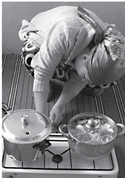
Figure 6: The cook verifies that the gas flames are exactly the same size under the two pots. This assures comparable energy use and would be difficult to realise precisely with a wood fire
