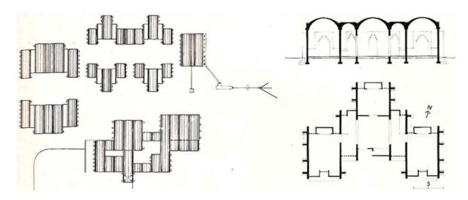
The Agricultural Training Center in Nianing, Senegal, completed in 1977, is a prototypical series of buildings based upon a relatively simple structural system of solid load bearing sand and cement block walls, parallel to one another and supporting shortspan barrel vaults. The vaults, whose thickness at the crown is only a little over 1½ inches, were formed using three layers of cement mortar stabilized with wire mesh at the top of the vault. As the construction photo (left)
