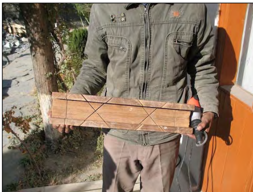
Mitre box of hardwood, an essential working tool for making precise joints.
