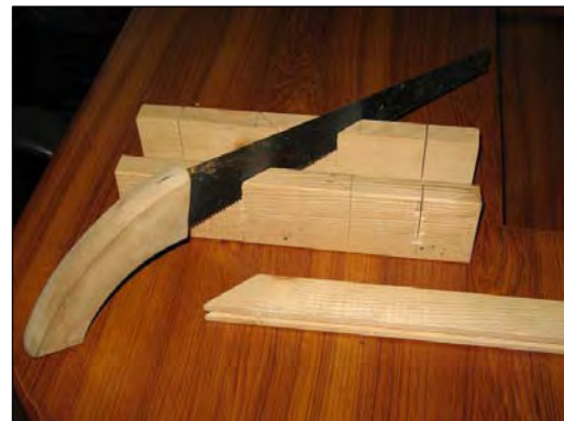
Mitre box of hardwood, an essential working tool for making precise joints.
