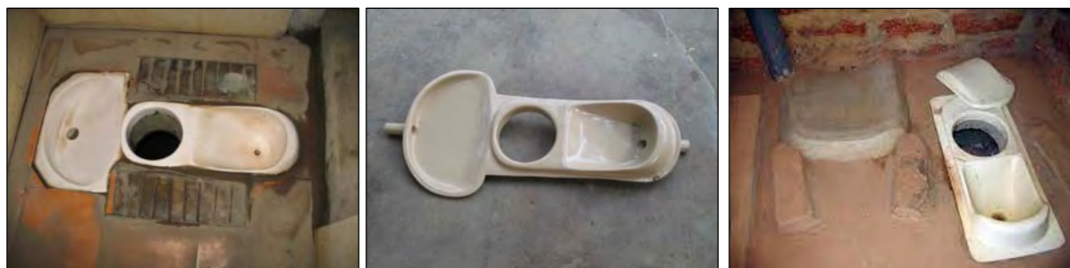
Left: Two section ceramic three-hole UDDT squatting pan that allows anal washing with water over the wider section (left), which goes separate into the “black water” drain. The drain on the right-hand side is for urine only, allowing the squat hole to remain dry.
