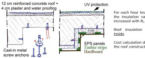
For each hour less than 5 hrs sun, the insulation value needs to be increased with  $R_c = 0.1 \text{ m}^2$ .K/W.
