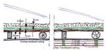
For each hour less than 5 hrs sun, the insulation value needs to be increased with  $R_c = 0.1 \text{ m}^2$ .K/W.
