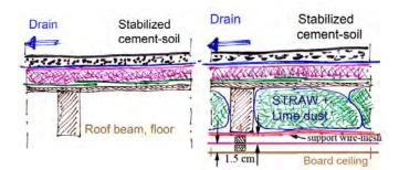
For each hour less than 5 hrs sun, the insulation value needs to be increased with  $R_c = 0.1 \text{ m}^2.\text{K/W}.$
