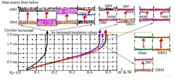
The red arrows indicate the direction of the heat flow.
