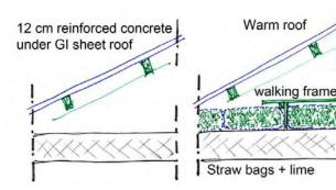
For each hour less than 5 hrs sun, the insulation value needs to be increased with  $R_{\rm C}=0.1\ m^2.K/W.$
