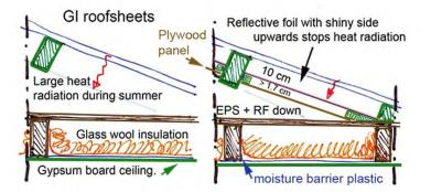
For each hour less than 5 hrs sun, the insulation value needs to be increased with  $R_c = 0.1 \text{ m}^2.\text{K/W}.$
