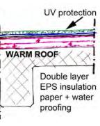
For each hour less than 5 hrs sun, the insulation value needs to be increased with  $R_c = 0.1 \text{ m}^2.\text{K/W}.$
