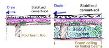
For each hour less than 5 hrs sun, the insulation value needs to be increased with  $R_{C}=0.1\ m^{2}.K/W.$
