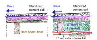
For each hour less than 5 hrs sun, the insulation value needs to be increased with  $R_{\rm C}=0.1\ m^2.K/W.$
