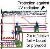
For each hour less than 5 hrs sun, the insulation value needs to be increased with  $R_c = 0.1 \text{ m}^2$ .K/W.
