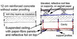
For each hour less than 5 hrs sun, the insulation value needs to be increased with  $R_c = 0.1 \text{ m}^2$ .K/W.
