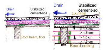
For each hour less than 5 hrs sun, the insulation value needs to be increased with  $R_{C}$  = 0.1  $m^{2}.K/W.$
