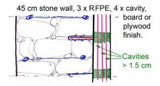
For each hour less than 5 hrs sun, the insulation value needs to be increased with  $R_{c}{=}$  0.1  $m^{2}{\rm .}K/W{\rm .}$
