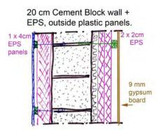
For each hour less than 5 hrs sun, the insulation value needs to be increased with  $R_{C}$  = 0.1  $m^{2}.K/W.$
