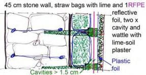
For each hour less than 5 hrs sun, the insulation value needs to be increased with  $R_c = 0.1 \text{ m}^2$ .K/W. Wall insulation applied on the inside.
