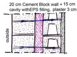
For each hour less than 5 hrs sun, the insulation value needs to be increased with  $R_c = 0.1 \text{ m}^2$ .K/W.
