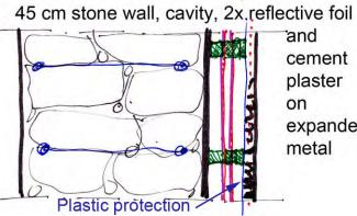
and cement plaster on expanded metal
