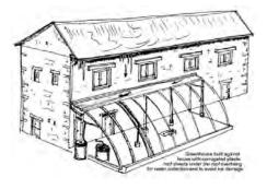
On the other hand, during sun hours, the sunlight entering the greenhouse will be converted into heat when it touches a building material. This heating will be faster when the surface is dark. The walls and floor area inside the greenhouse will be heated up and will serve as a heat storage. The warmed-up walls and floor will later release the stored heat when the sun disappears.
