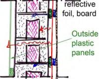
For each hour less than 5 hrs sun, the insulation value needs to be increased with  $R_{\rm C}$  = 0.1  $m^2.K/W.$
