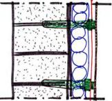
For each hour less than 5 hrs sun, the insulation value needs to be increased with  $R_c = 0.1 \text{ m}^2$ .K/W.
