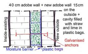
For each hour less than 5 hrs sun, the insulation value needs to be increased with  $R_{c}$  = 0.1  $m^{2}.K/W.$
